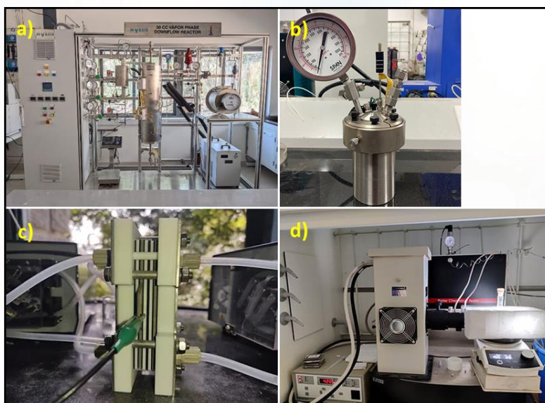
Figure 1: a) Fixed bed continuous flow reactors b) Batch reactor c) Electrochemical flow cell setup d) Photochemical reaction setup. (Images are taken from JNCASR, Bangalore's website.)
